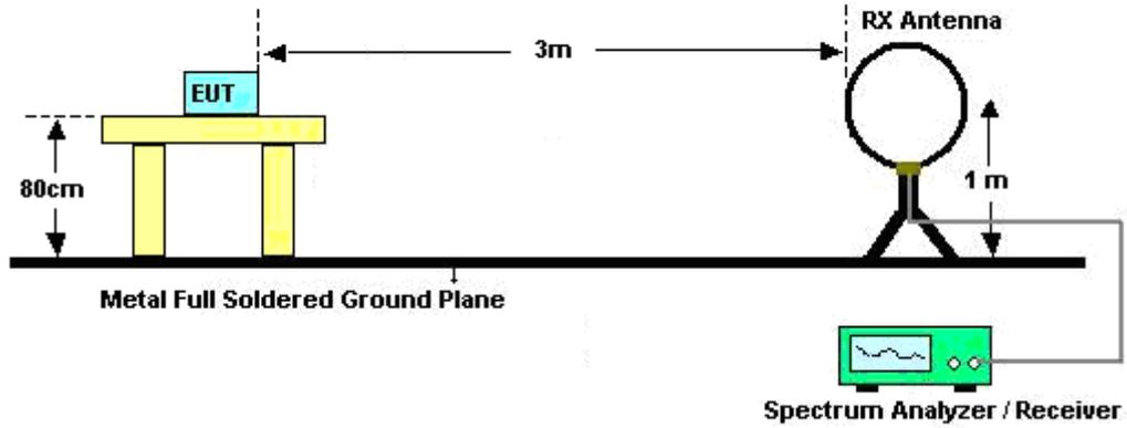
For radiated emissions from 30MHz to 1GHz
