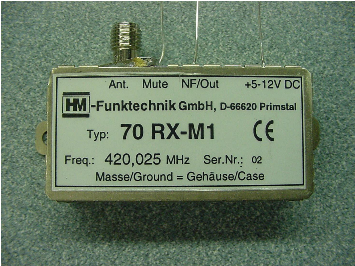
PHOTOGRAPH 3: FRONT VIEW OF RECEIVER
