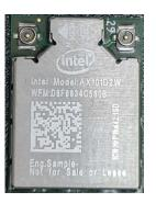
Note: Due to the small device size 12mm x 16mm it is too small to imprint the FCCID and IC ID on the module. The font size required would need to be < size 4 font and is considered to require magnification for legibility. The ID's will be placed in the Information Guide. External host labeling is still required once integrated into host.
