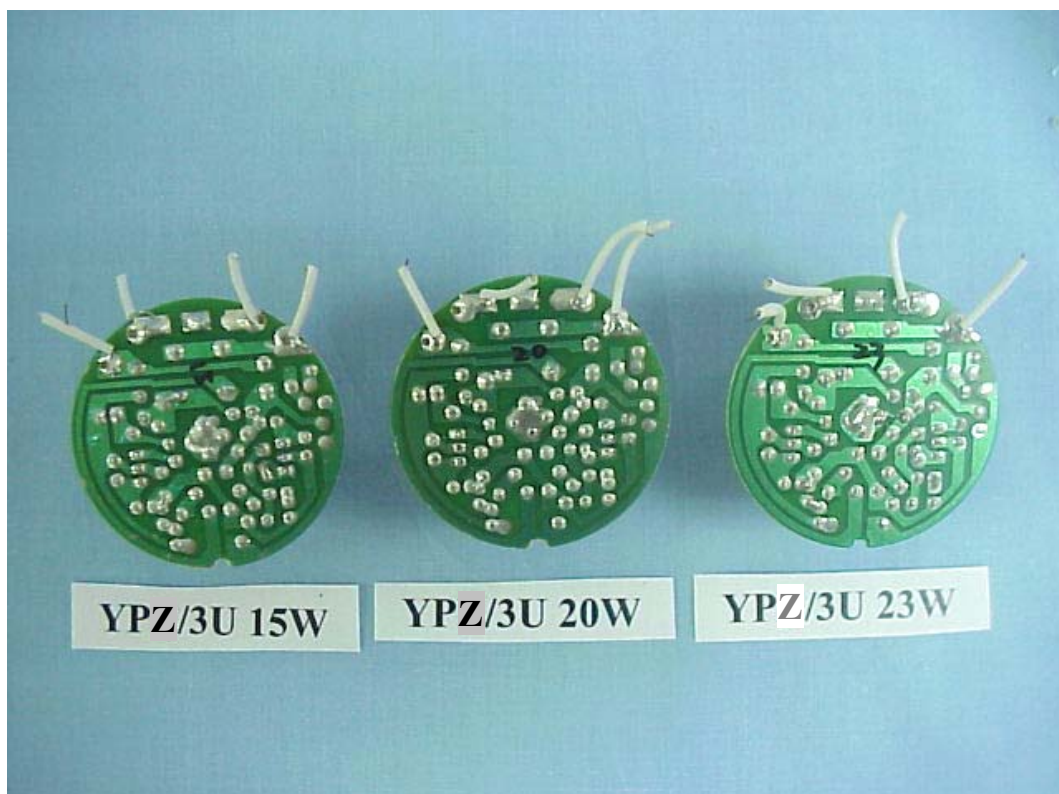
FIGURE 3 ENERGY SAVING LAMP (M/N: YPZ/3U 15W/20W/23W) MAIN BOARD (SOLDERED SIDE)
