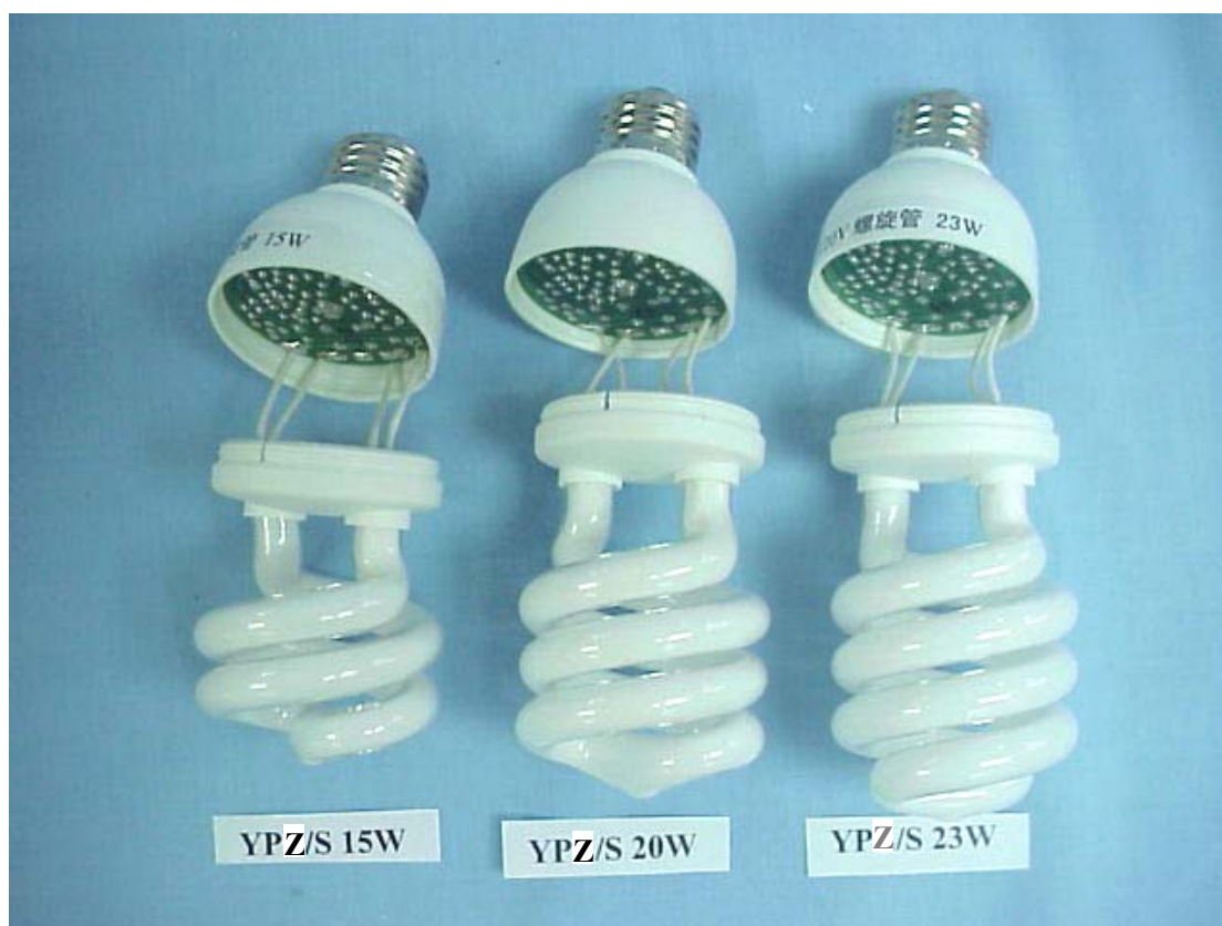
FIGURE 4 ENERGY SAVING LAMP (M/N: YPZ/S 15W/20W/23W) COVER REMOVED
