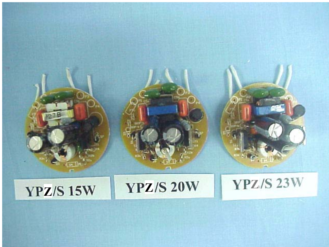
FIGURE 5 ENERGY SAVING LAMP (M/N: YPZ/S 15W/20W/23W) MAIN BOARD (COMPONENT SIDE)
