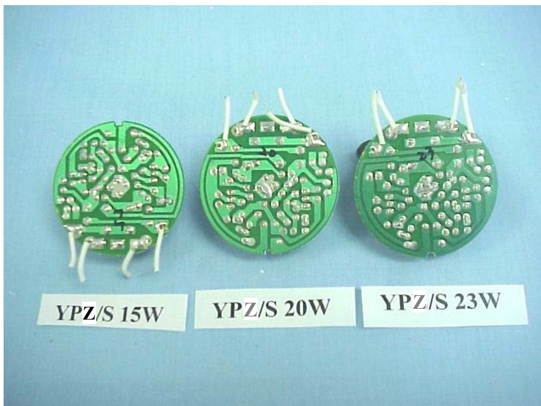
FIGURE 6 ENERGY SAVING LAMP (M/N: YPZ/S 15W/20W/23W) MAIN BOARD (SOLDERED SIDE)
