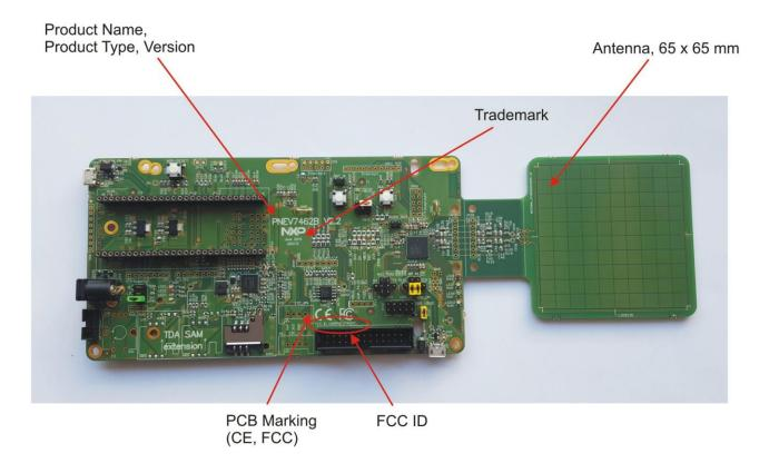
PCB Marking and Label for PN7462AU Customer Demo Board, PNEV7462B V2.2 with FCC ID: OWRPNEV7462B
