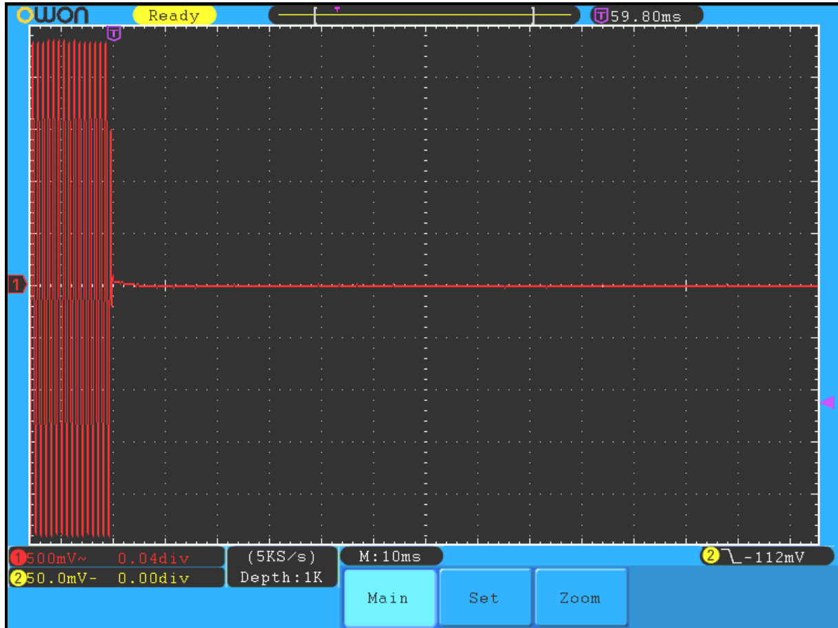
Plot 10-1: Transient Frequency Behavior – 430.0125 MHz; Wide Band; Carrier ON Time
