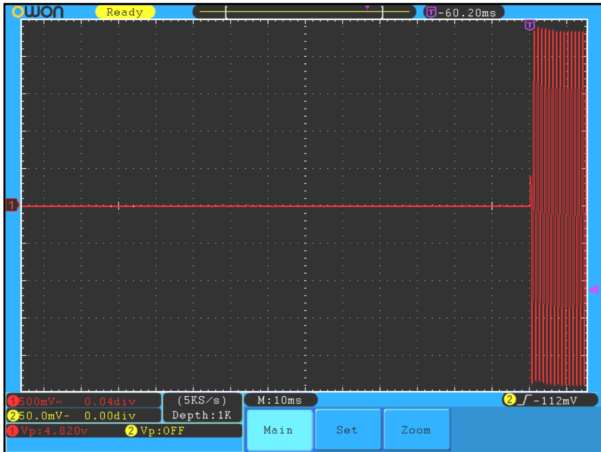
Plot 10-10: Transient Frequency Behavior – 511.9875 MHz; Wide Band; Carrier OFF Time
