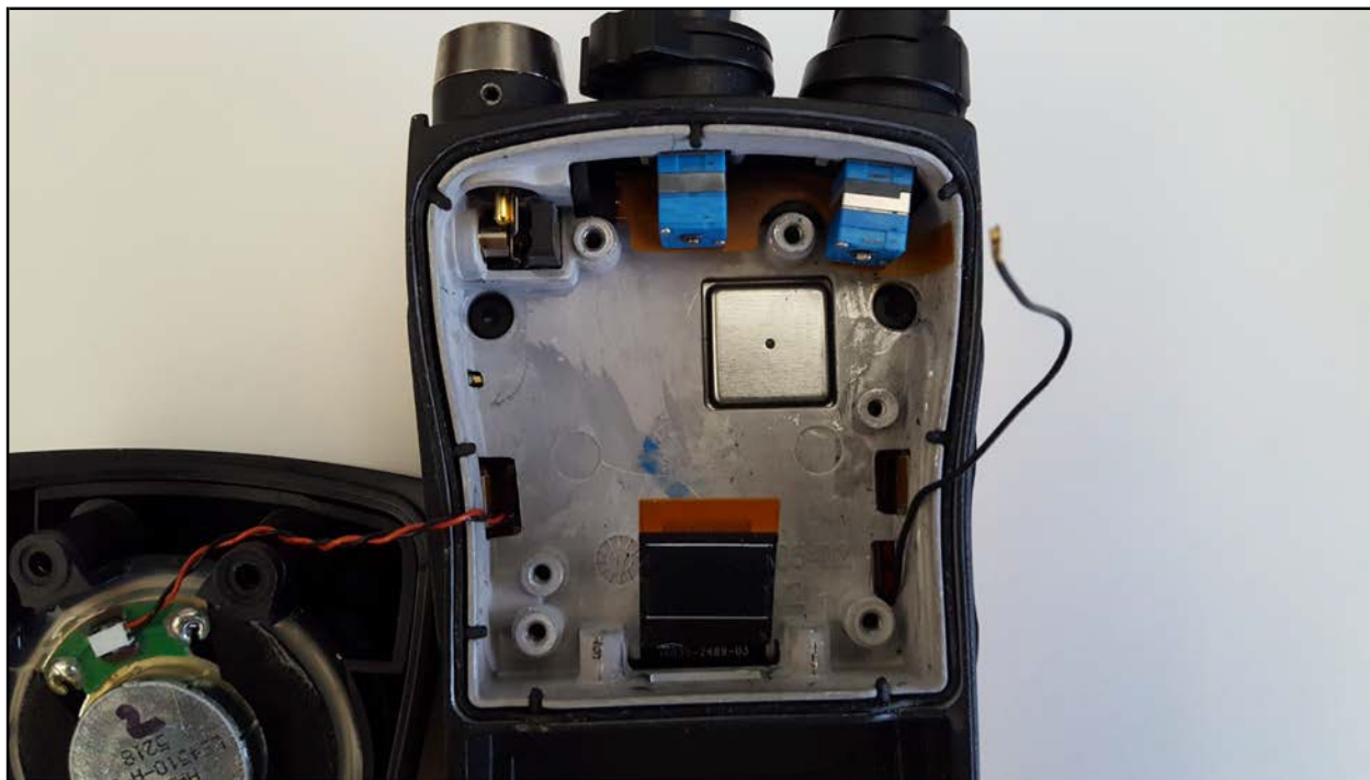
Rear Cover and Expansion Board Removed
