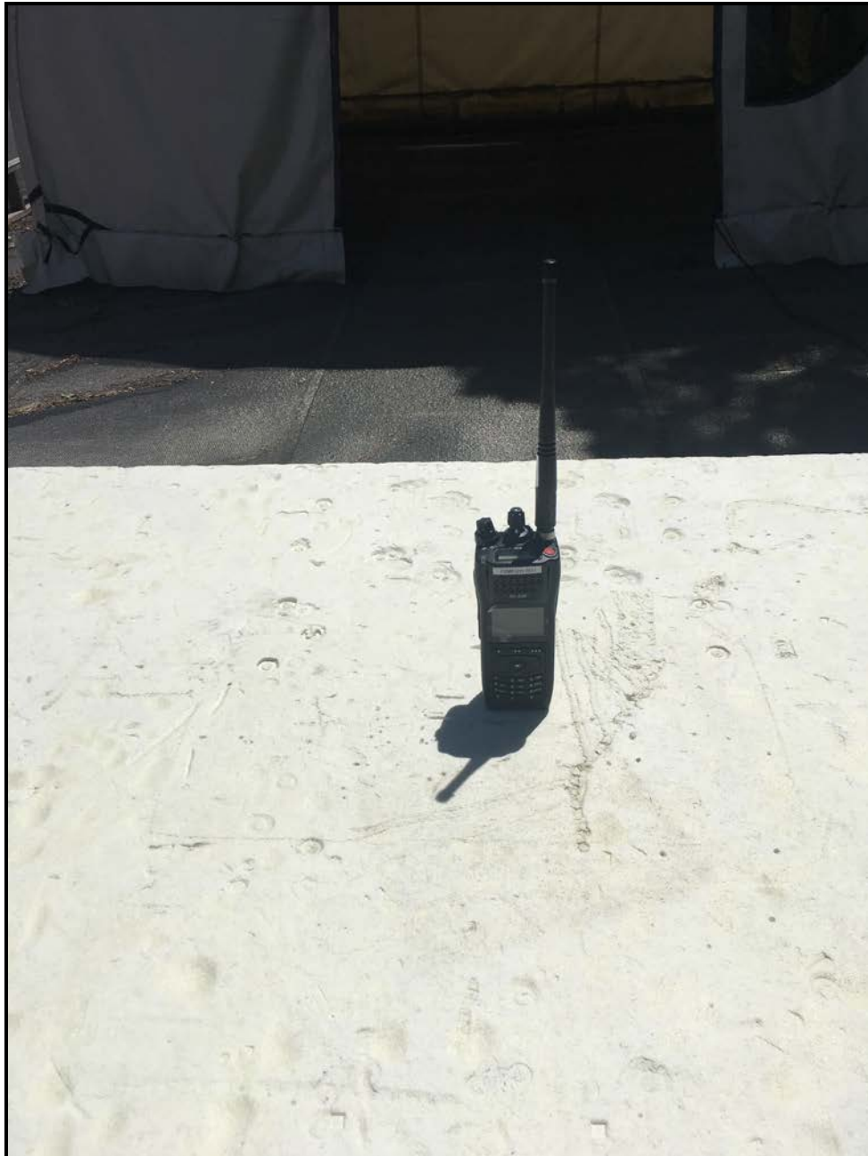
Photograph 3: Radiated Emissions (Spurious/Harmonics) Under 1 GHz, Front View
