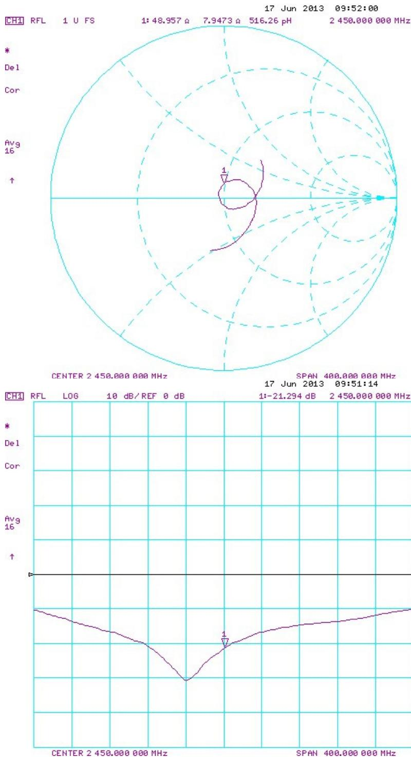
**2450 MHz Dipole Extended Calibration****Antenna VSWR with Head TSL**
