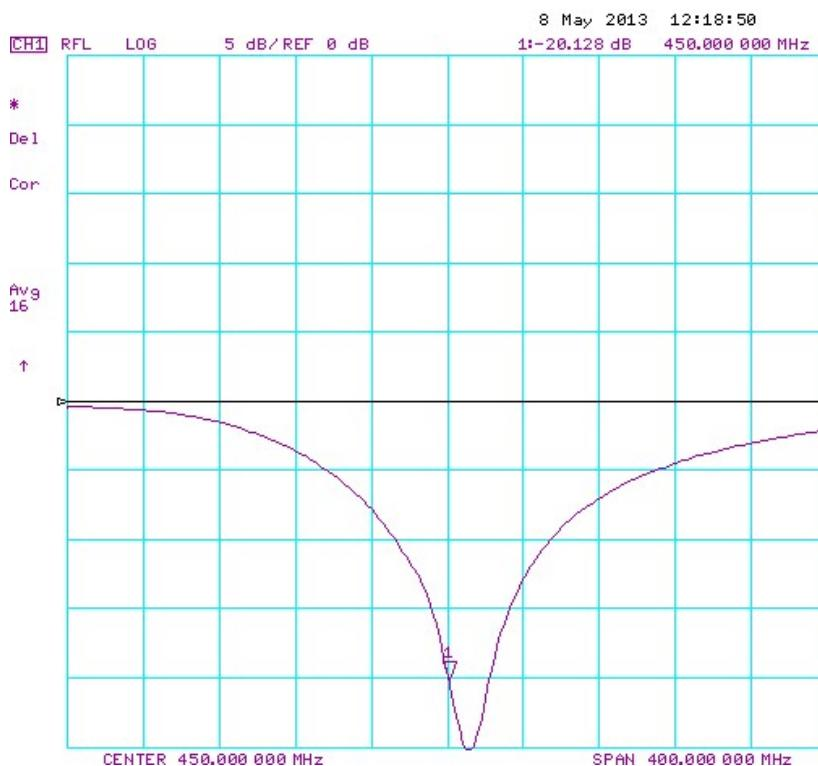
**450 MHz Dipole Extended Calibration**
