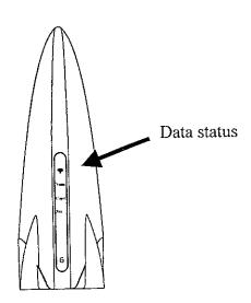
4. Point the keyboard to the receiver within a distance of 1 feet and press any of following keys simultaneously. The "data status" LED will blink once. Now, the operation channel is no change, and, one ID code is change. You can use the wireless keyboard now!
