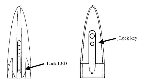
3. How to do the initial setting. Release the "lock" key, the "lock LED" will light off. Press the "CH", "ID" and "r" simultaneously. The keyboard will be on default setting or factory setting (channel 1 and ID 1).
