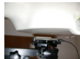
Figure 14.9 Body SAR Test Setup -- w/o Belt-clip --
