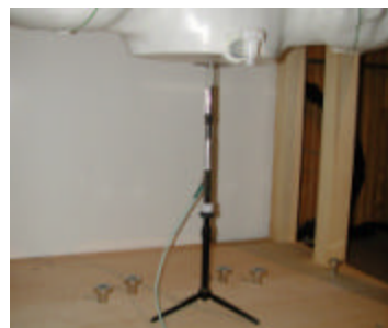
Figure 12.1 Dipole Validation Test Setup
