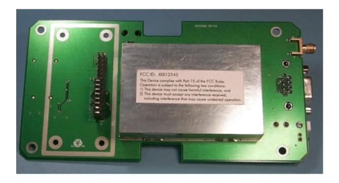
Figure E7.2. Photograph of DTSA showing FCC Identifier label placement.
