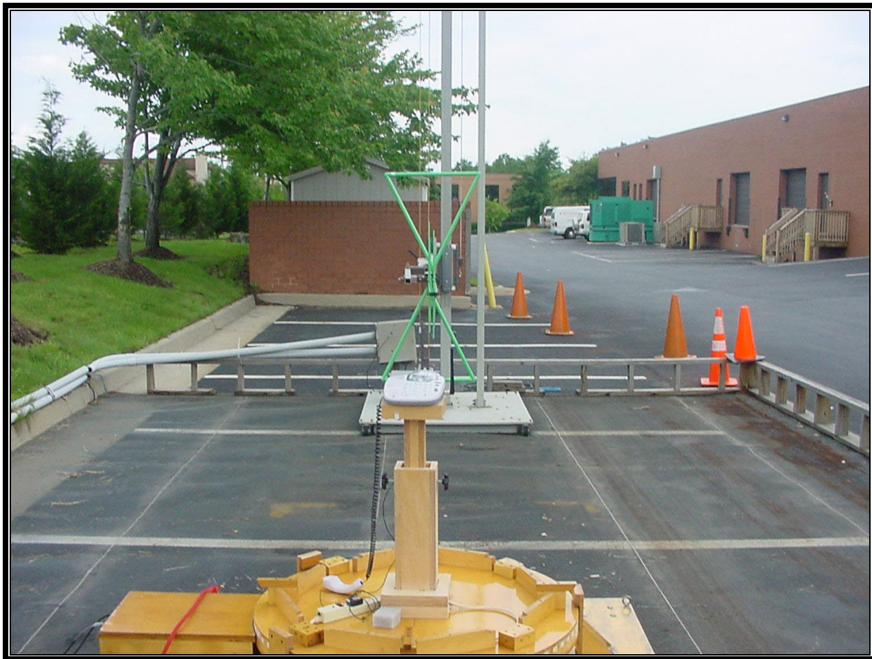
PHOTOGRAPH 2: RADIATED FRONT VIEW WITH WHIP ANTENNA
