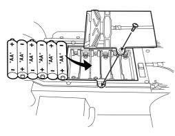
With parental supervision, unscrew top of battery compartment beneath the vehicle. Then, place 6 (six) AA alkaline batteries inside & re-screw top closed.
