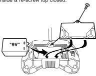
With your parent's help, unscrew top to battery compartment on remote control. Then, place 1(one) 9-Volt battery inside and re-screw top closed.
