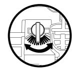
7. Turn the wheel alignment switch (located towards the front end of the vehicle) to initially line up the Sewer Spewer's direction, either in the middle, to the left, or to the right.
