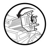
Shake Sewer Spew canister well before use. Then, place the Sewer Spew canister into the main turret body cavity with the top of the canister facing out.
