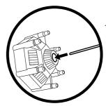
10. Shake Sewer Spew canister well before use. In case of jam-up or prolonged inactivity, clean nozzle with sharp object and shake well again. Sewer Spewer can be refilled with Sewer Spew.
