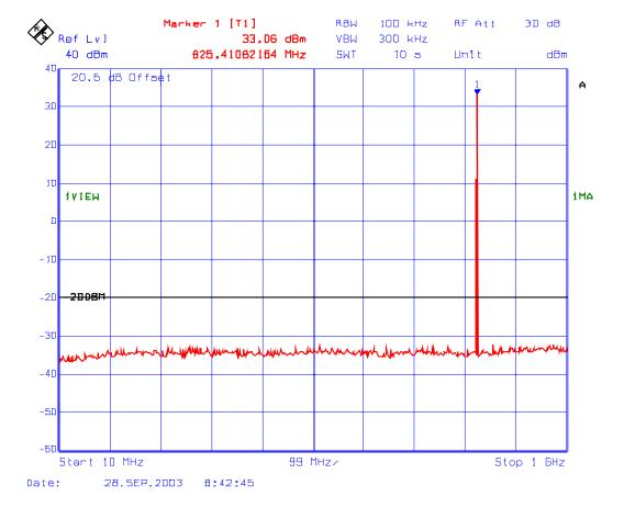
Plot # 31: Transmitter Spurious Conducted Emissions
