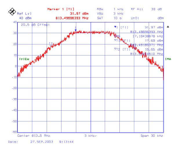
Plot #4: 99% Bandwidth in 806-821 MHz Band (25 kHz Channel Spacing) Frequency: 821 MHz, Modulation: 4-Level FSK RDLAP 19.2 kbps
