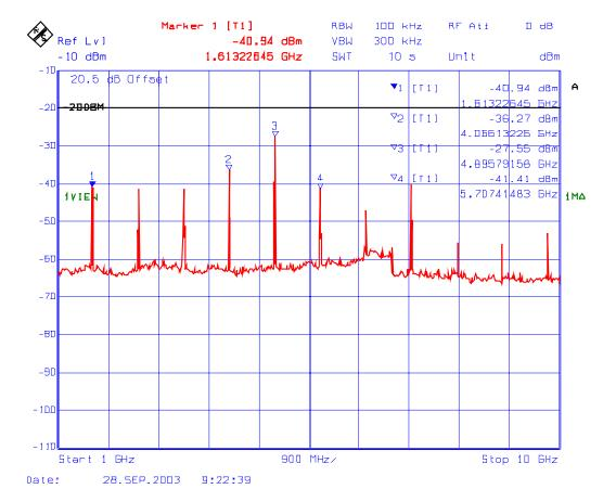
Plot # 24: Transmitter Spurious Conducted Emissions Frequency: 224 MHz, Power Output: 0.5 Watts (Low) Modulation: 4-Level FSK RDLAP 9.6 kbps
