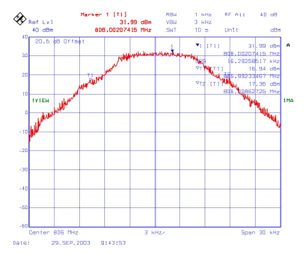
Plot #3: 99% Bandwidth in 806-821 MHz Band (25 kHz Channel Spacing) Frequency: 813.5 MHz, Modulation: 4-Level FSK RDLAP 19.2 kbps
