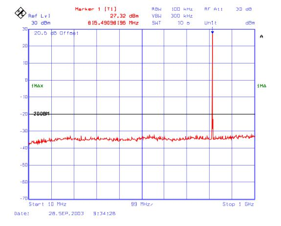
Plot # 23: Transmitter Spurious Conducted Emissions
