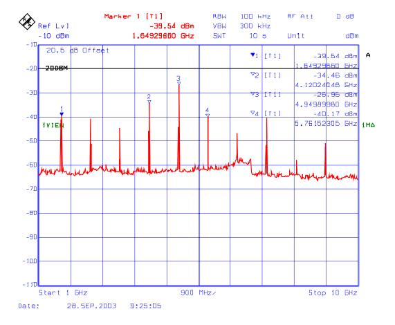
Plot # 26: Transmitter Spurious Conducted Emissions
