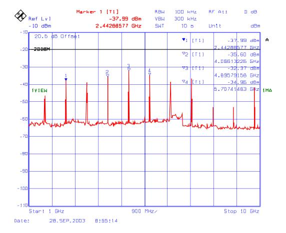
Plot # 30: Transmitter Spurious Conducted Emissions
