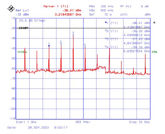
Plot # 22: Transmitter Spurious Conducted Emissions Frequency: 815 MHz, Power Output: 0.5 Watts (Low) Modulation: 4-Level FSK RDLAP 19.2 kbps
