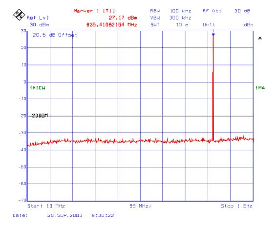
Plot # 25: Transmitter Spurious Conducted Emissions Frequency: 824 MHz, Power Output: 0.5 Watts (Low) Modulation: 4-Level FSK RDLAP 9.6 kbps
