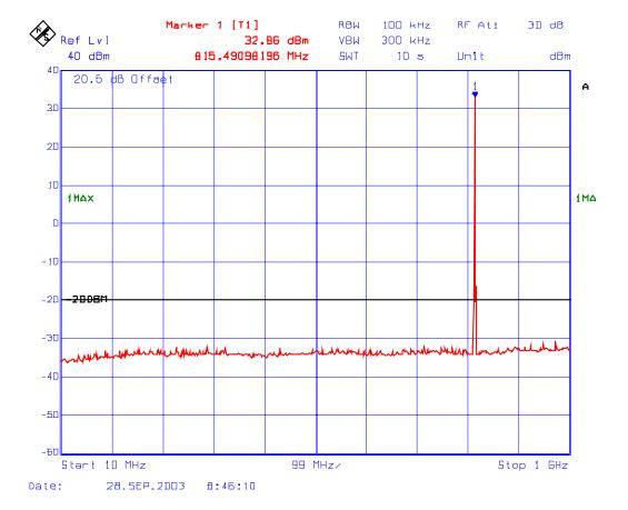
Plot # 29: Transmitter Spurious Conducted Emissions
