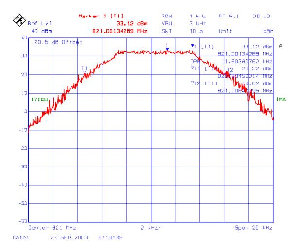
Plot #6: 99% Bandwidth in 821-824 MHz Band (12.5 kHz Channel Spacing) Frequency: 822.5 MHz, Modulation: 4-Level FSK RDLAP 9.6 kbps
