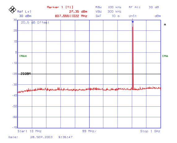
Plot # 21: Transmitter Spurious Conducted Emissions
