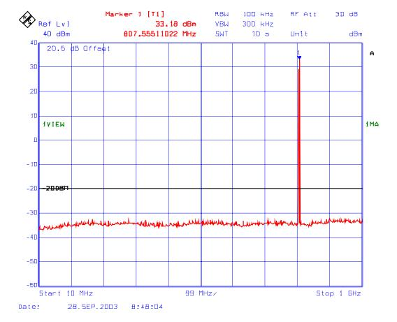
Plot # 27: Transmitter Spurious Conducted Emissions
