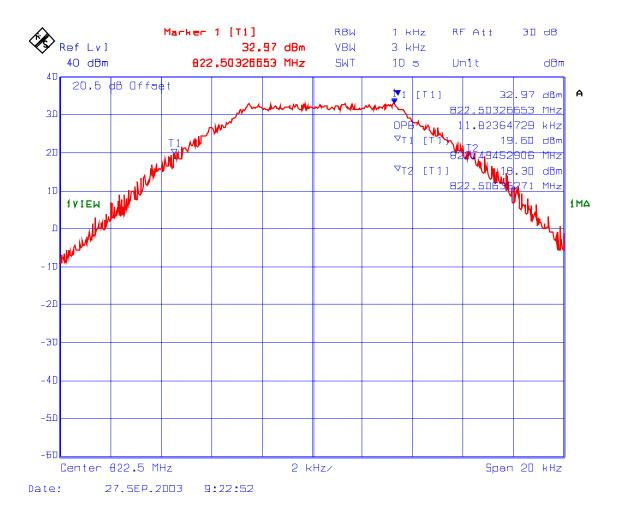
Plot #7: 99% Bandwidth in 821-824 MHz Band (12.5 kHz Channel Spacing) Frequency: 824 MHz, Modulation: 4-Level FSK RDLAP 9.6 kbps
