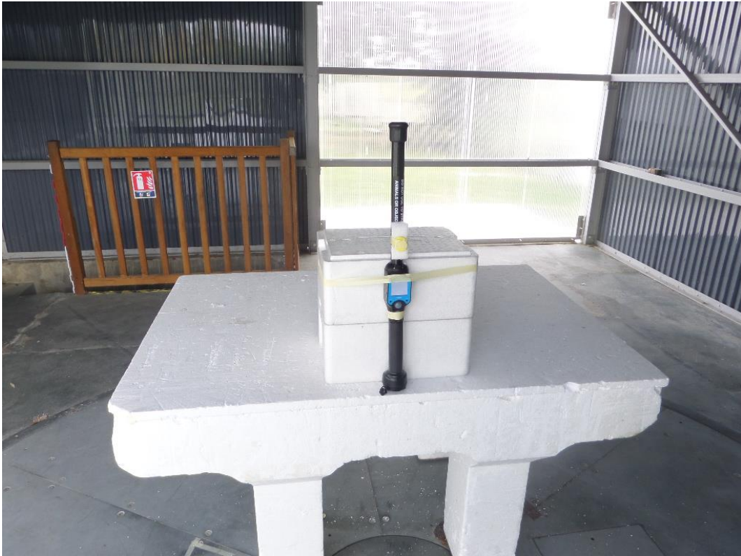
Open Area Test Site RFID in Position 1 with battery
