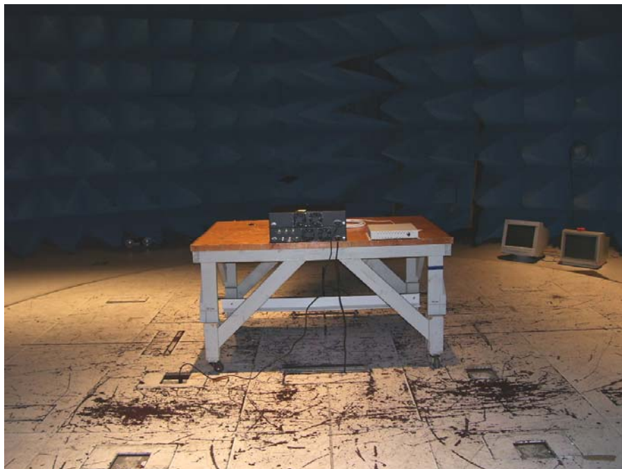
Photograph 6. Radiated Emission Limits Test Setup, 30 MHz to 1 GHz, Back View
