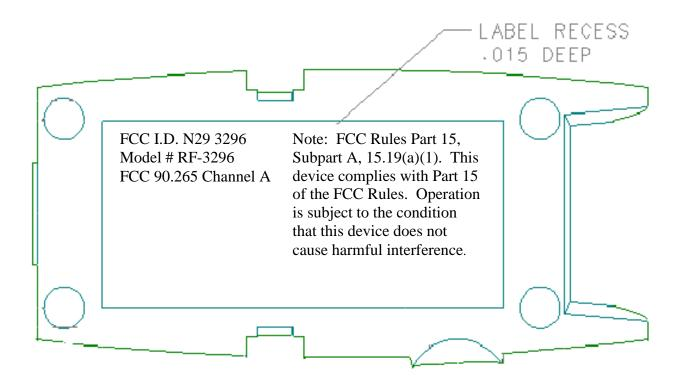
The following is a drawing of the side of the headset showing the FCC ID label and the FCC ID label location. The FCC warning text appears in a prominent location in the manual as the product is too small to accommodate the text.
