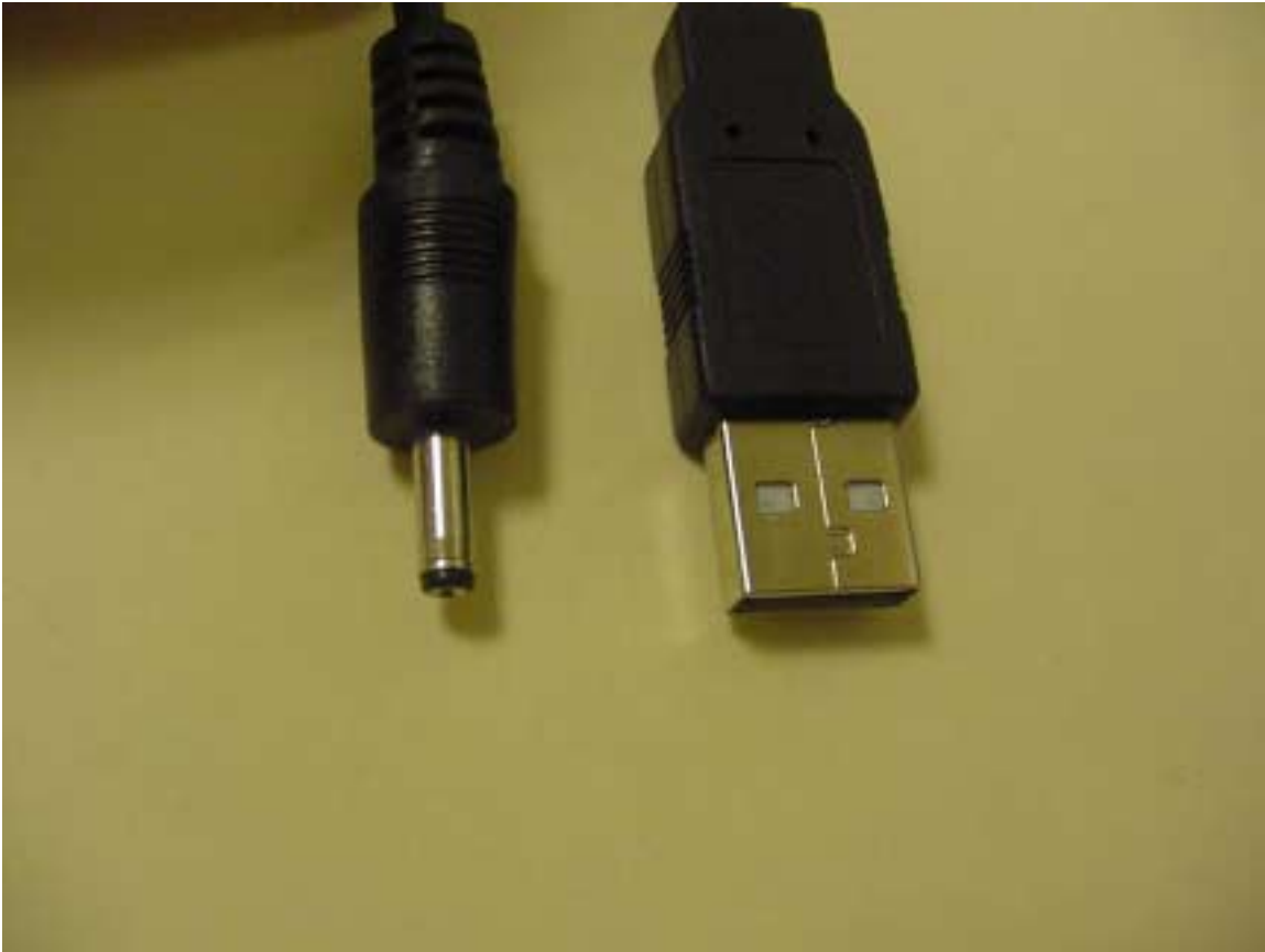
USB Cable connectors, standard USB on the right and a simple power connector on the left.
