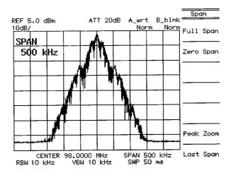
The FCC rule 73.317 limits the emission between 120kHz and 240kHz from the carrier frequency to -25 dB, between 240kHz and 600kHz to -35 dB and for higher frequency than 600kHz the emission may be at least 43+10 log  $P_o$ , or -67 dB referenced to the unmodulated carrier. In the stereophonic mode the emissions are below the limits.
