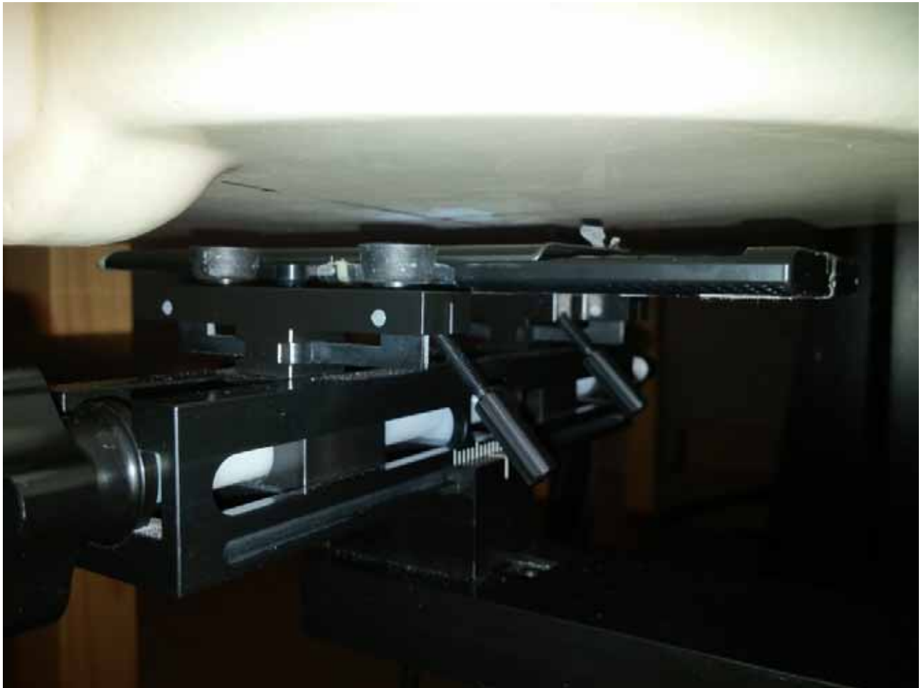
Figure E12. Hotspot configuration – Slider Open (No Holster, front side 10mm away)
