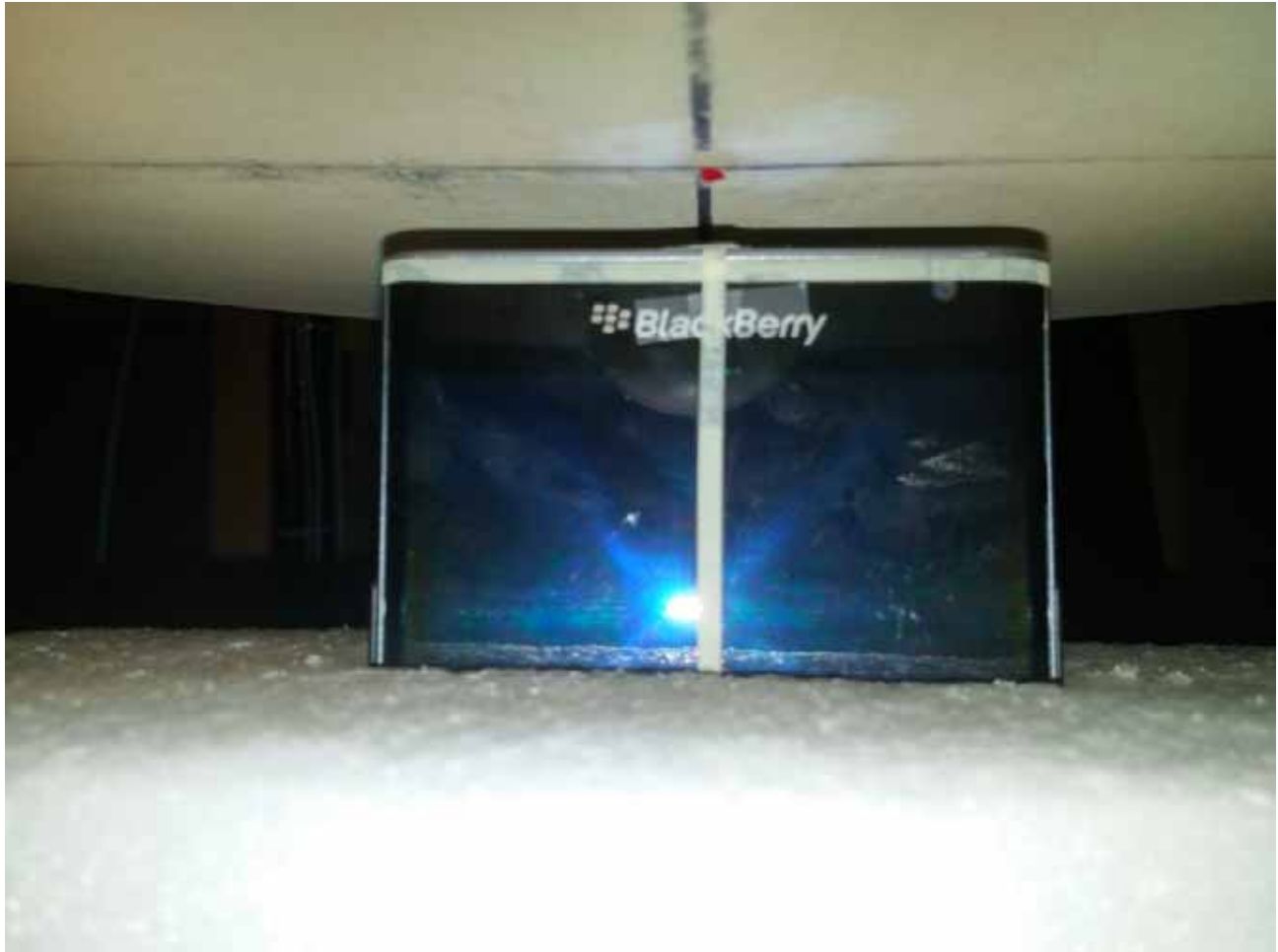
Figure E18. Hotspot configuration – Slider Open (No Holster, top side 10mm away)
