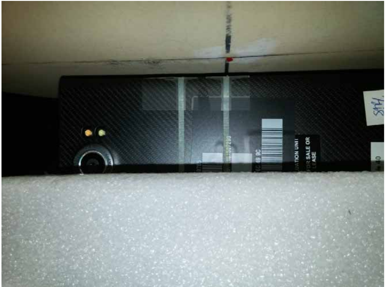
Figure E13. Hotspot configuration – Slider Closed (No Holster, left side 10mm away)
