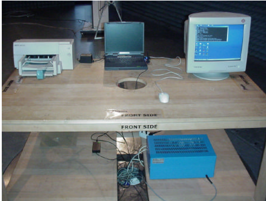
Picture 1 : Setup for the test "radiated emission"
