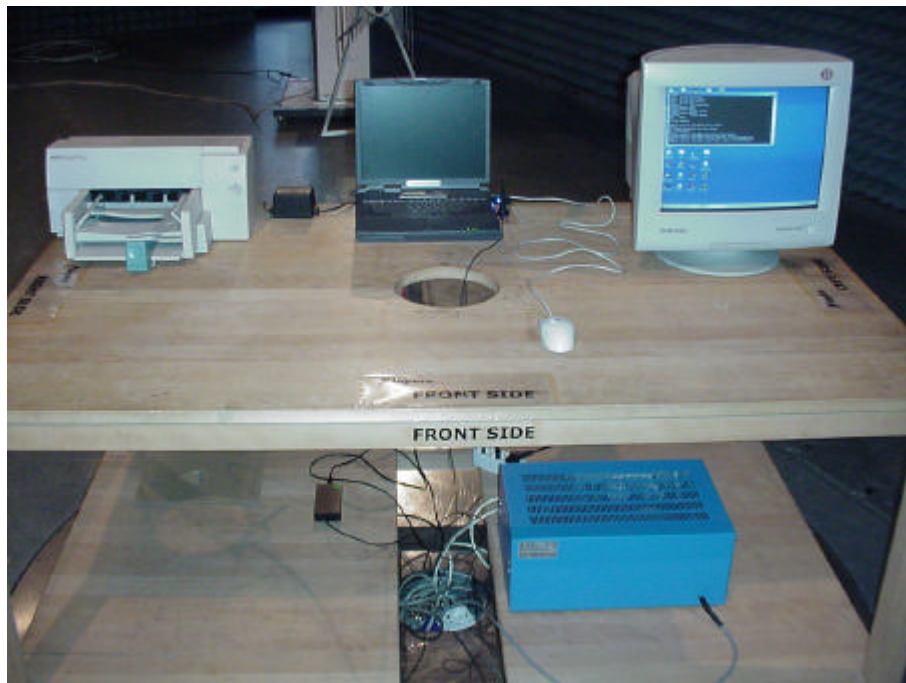
Picture 1 : Setup for the test "radiated emissions"
