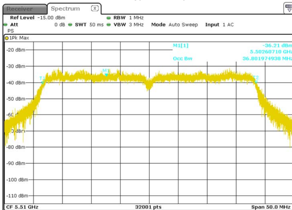
U-NII 99% Channel bandwidth
