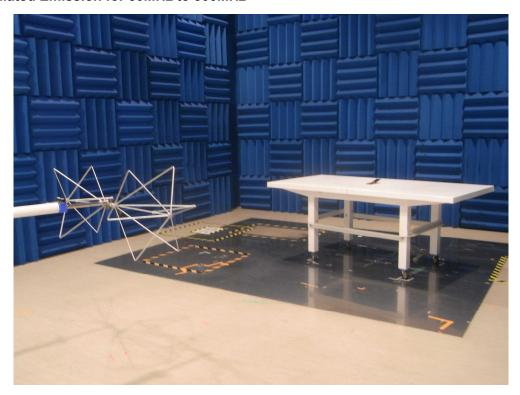
Radiated Emission for 300MHz to 1GHz
