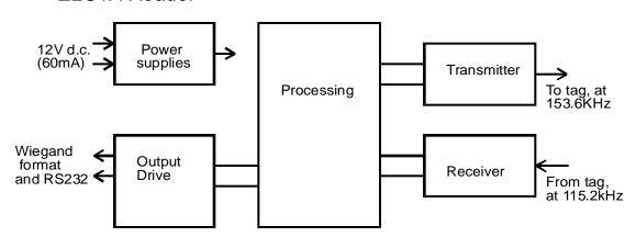
The ELC1A reader is a totally self-contained reader which is part of the Cryptag Census product range. It is 213mm by 163mm, and apart from the area containing the terminal block it is only 4.5mm thick.
