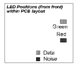
To check that the reader is working, apply power to the reader. The red LED should come on, as also should the Data LED. The Noise LED should be off. Bring a tag in towards the reader. Three things should happen.
