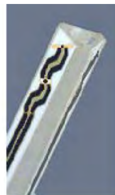
Figure 2.3 Probe Thick-Film Technique
