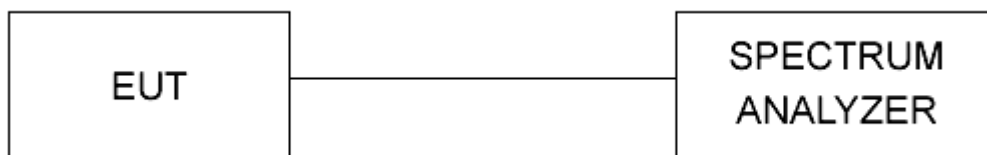
Figure 1 - Bandwidth Measurements Test Setup
