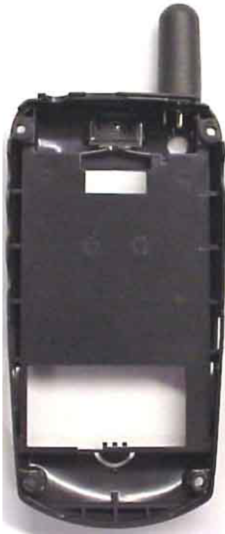
Rear Housing Internal View
