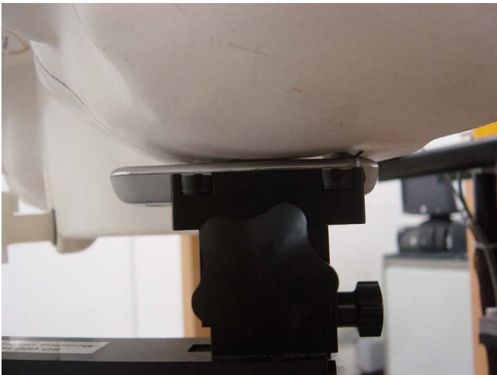
Figure 4. Phone Against the Head Phantom (Cheek Touch)
