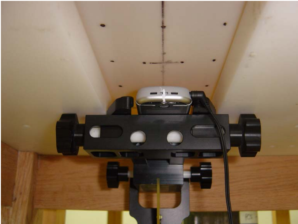
Figure 3. Phone Against the Flat Phantom
