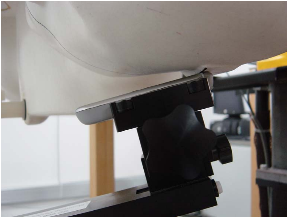
Figure 5. Phone Against the Head Phantom (15°Tilt)
