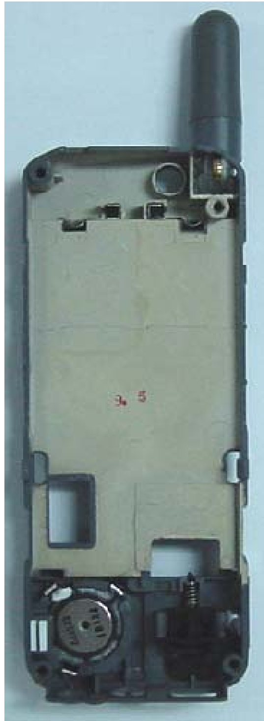
Rear Housing (Internal View)
