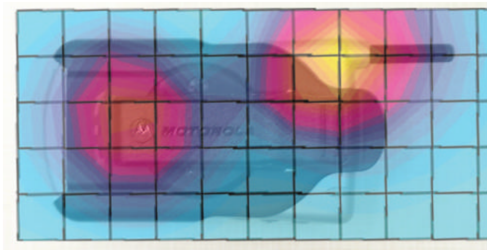
Figure 8. Typical 1900MHz with Antenna Retracted Contour Plot Overlaid on Body Worn Accessory
