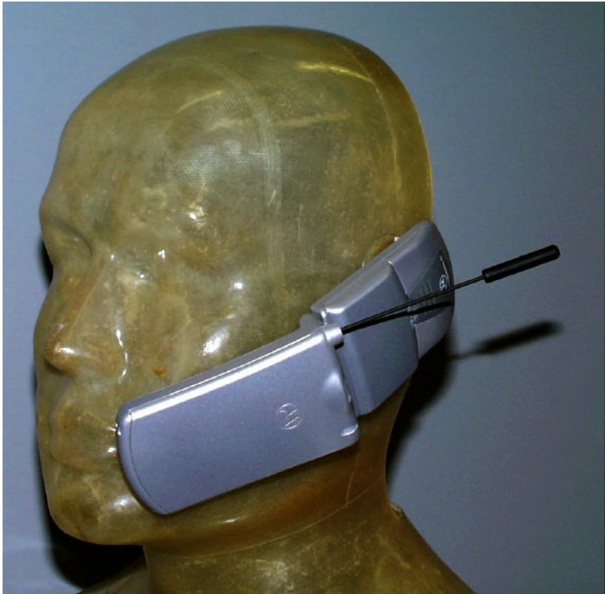
Figure 15. Phone against Head Phantom with Antenna Extended
