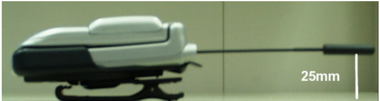
Figure 9. Separation Distance Provided by Body Worn Accessory with Antenna Extended.
