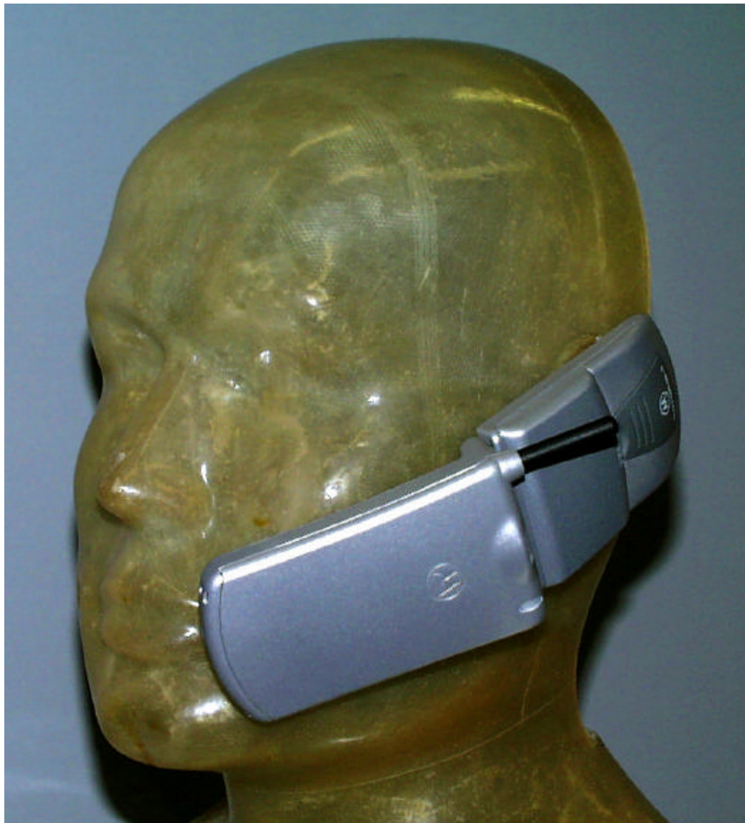
Figure 16. Phone against Head Phantom with Antenna Retracted
