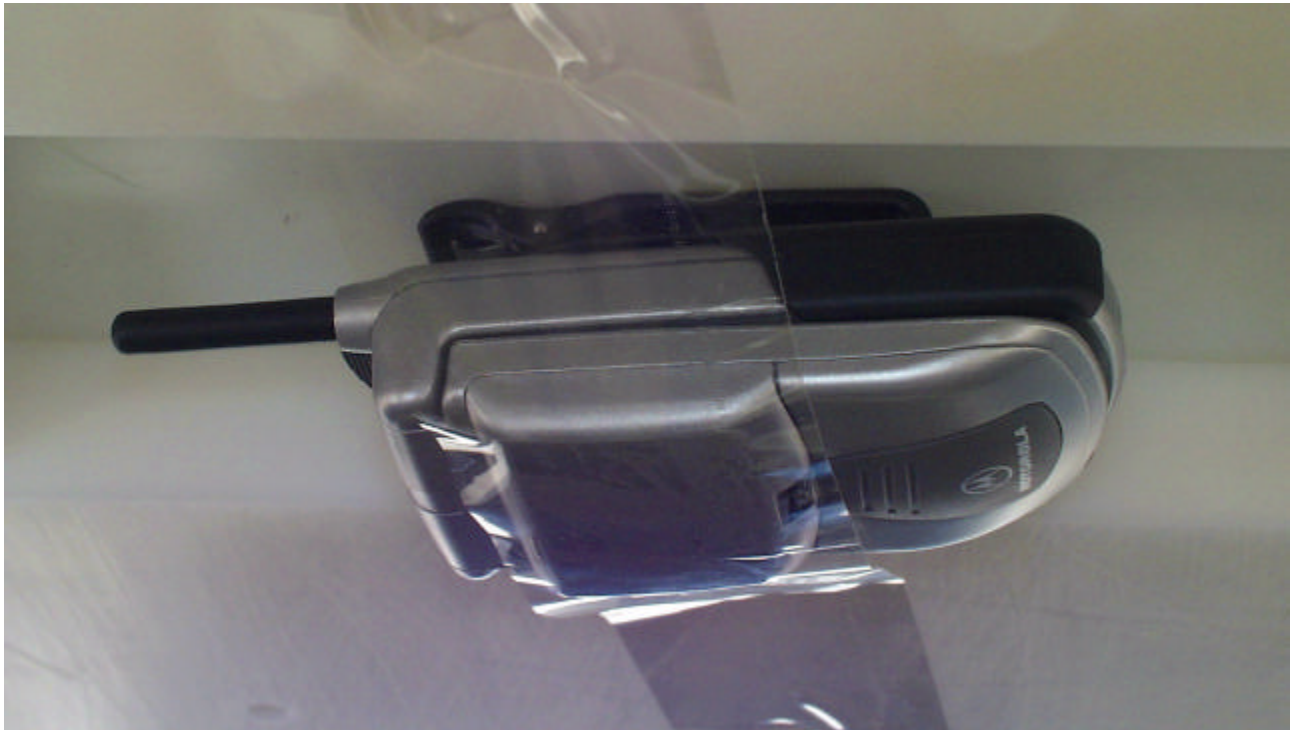
Figure 14. Phone in Supplied Belt Clip against Phantom
