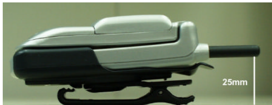
Figure 10. Separation Distance Provided by Body Worn Accessory with Antenna Retracted.
