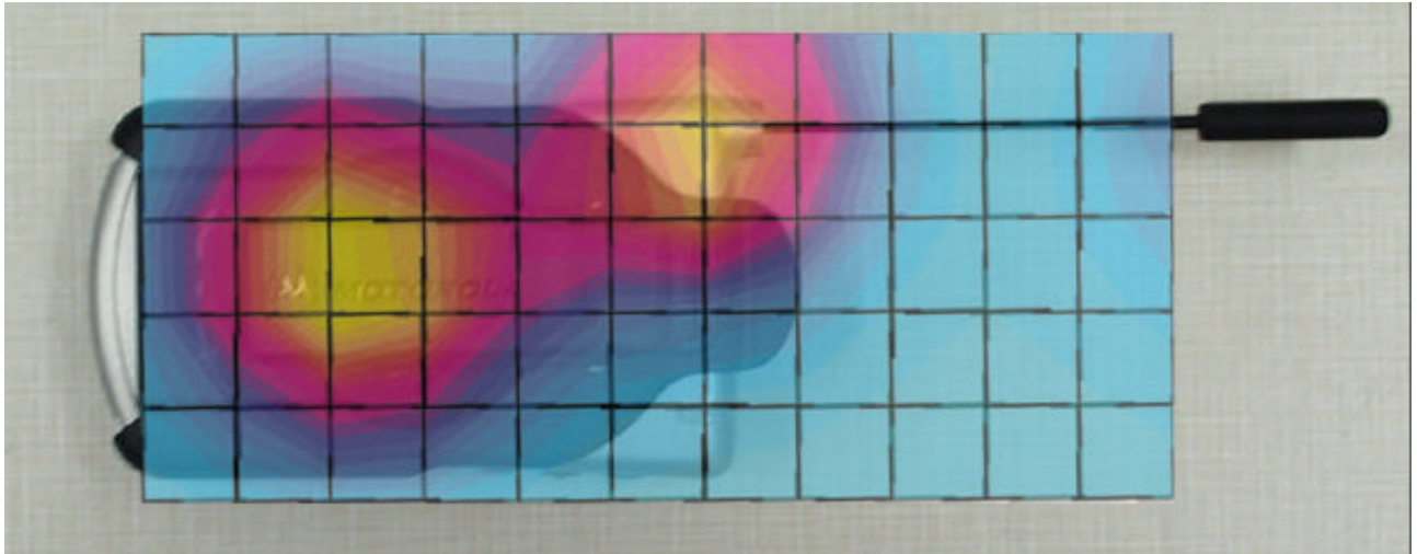
Figure 7. Typical 1900MHz CDMA with Antenna Extended Contour Plot Overlaid on Body Worn Accessory
