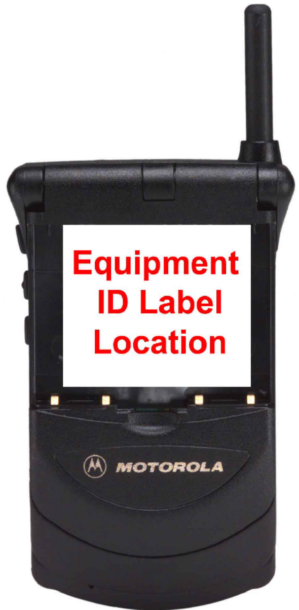
Flip Closed & Battery Removed to Show Equipment ID
