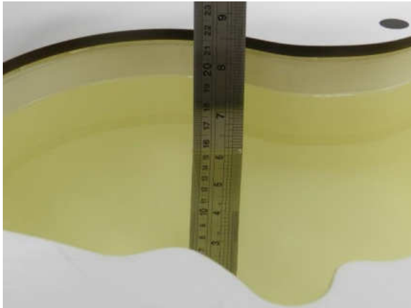
Fig 10.1 Photo of Liquid Height for Head SAR
