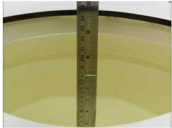
Fig 10.2 Photo of Liquid Height for Body SAR
