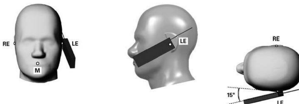
Fig 9.3.1 Tilt position. The reference points for the right ear (RE), left ear (LE), and mouth (M), which define the Reference Plane for handset positioning, are indicated.
