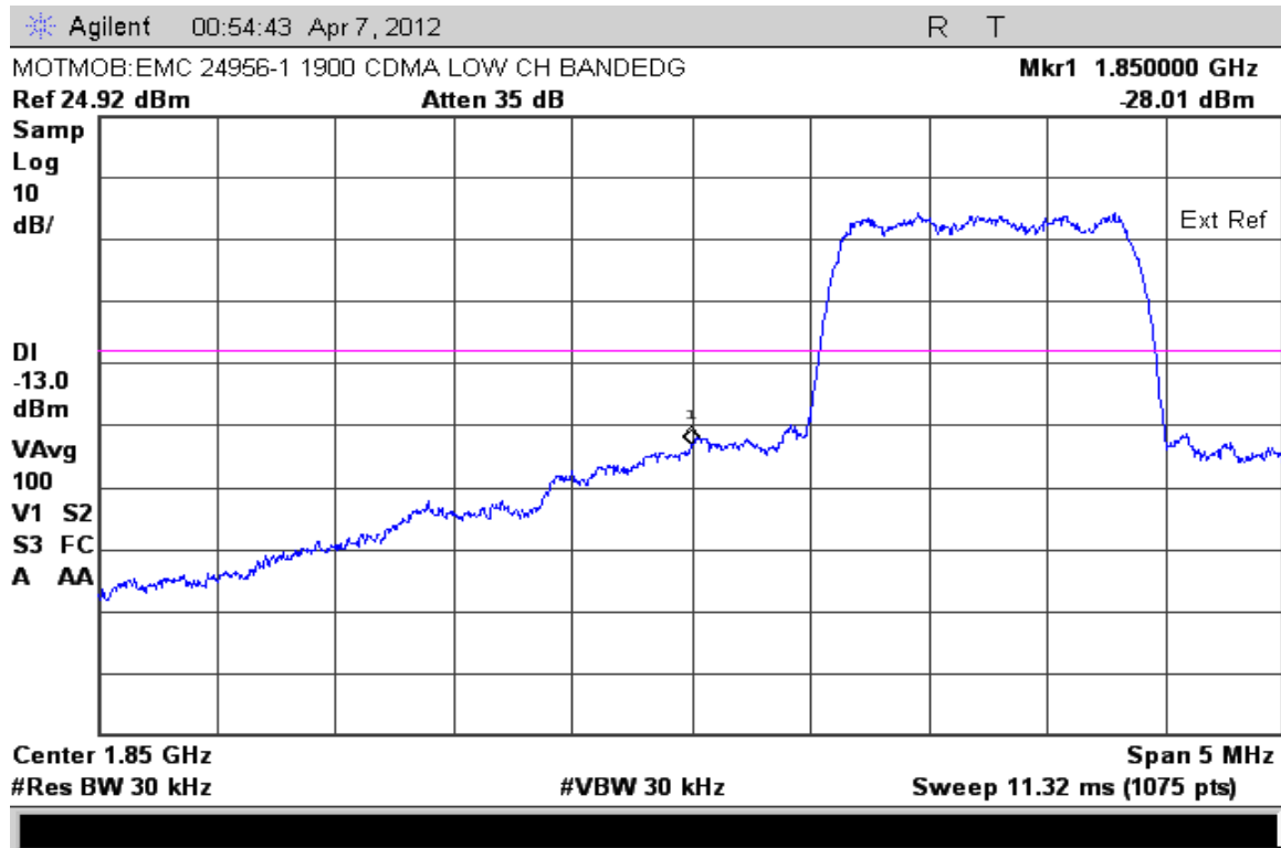
CDMA 1900 – Lower Band Edge – Channel 25 (1851.25MHz)
