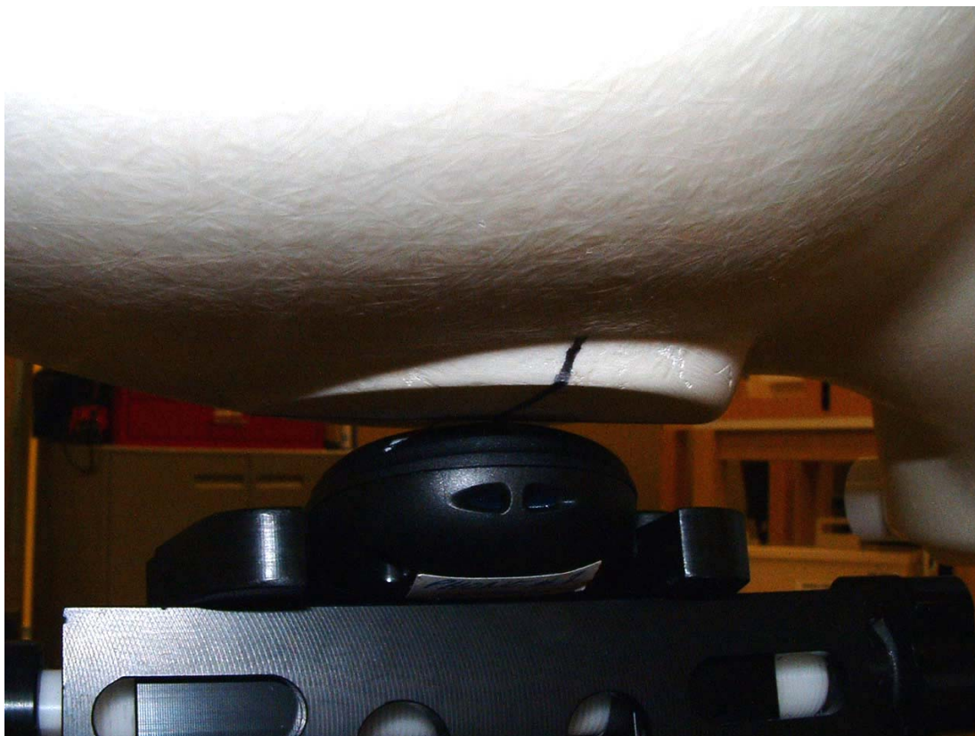
Figure 7. Phone Against the Head Phantom (Back View – 15°Tilt)
