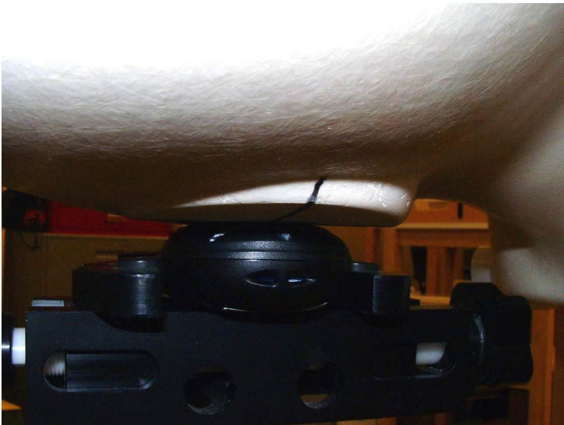
Figure 5. Phone Against the Head Phantom (Back View – Cheek Touch)
