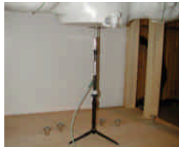
Figure 12.1 Dipole Validation Test Setup
