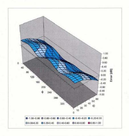
Spherical Isotropy Error < ± 0.4 dB
