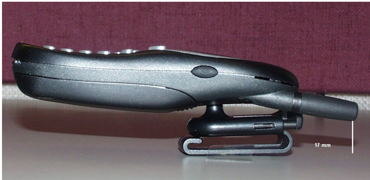
Figure 16. Distance of the Antenna (Retracted) to the Base of the Flat Phantom (17 mm)
