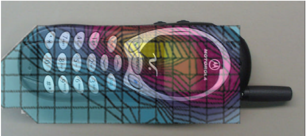
Figure 3. Typical 800MHz Head Adjacent Contour Overlaid on Phone with Antenna Retracted
