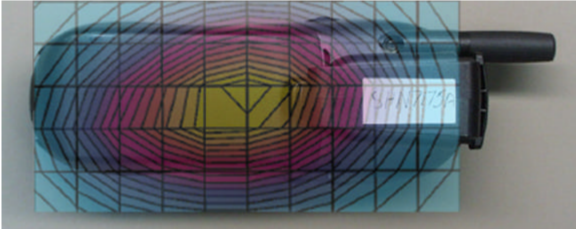
Figure 5. Typical 800 MHz Body-Worn Contour Overlaid on Phone with Antenna Retracted
