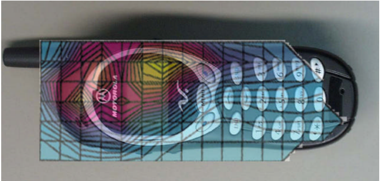
Figure 1. Typical 1900MHz Head Adjacent Contour Overlaid on Phone with Antenna Retracted
