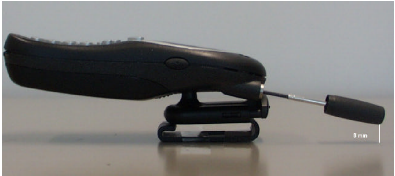
Figure 15. Distance of the Antenna (Extended) to the Base of the Flat Phantom (8mm)
