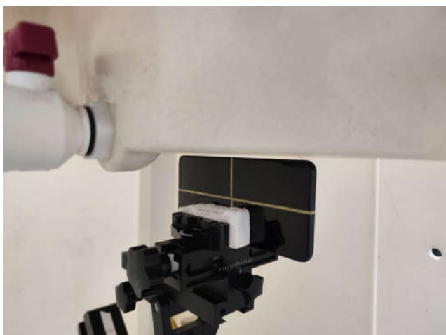
Left Side, Test Separation 3 mm
