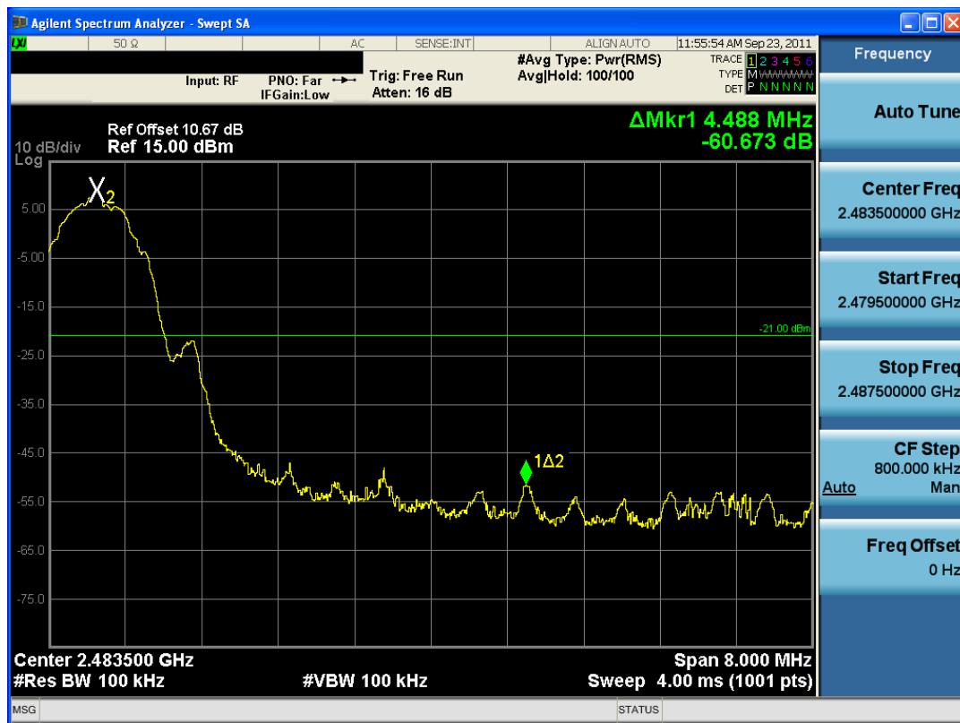
Plot 6-8. Band Edge Plot (Bluetooth (LE) – Ch. 39)
