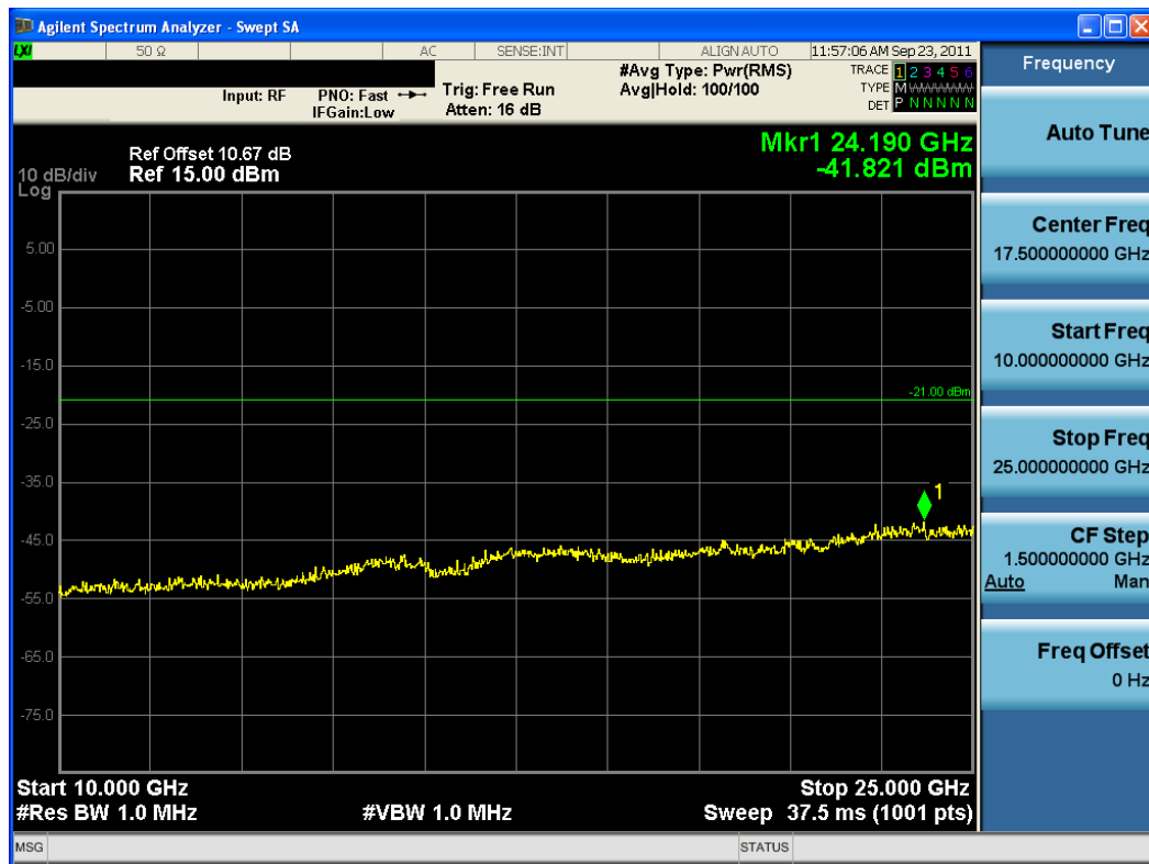
Plot 6-14. Conducted Spurious Plot (Bluetooth (LE) – Ch. 39)
