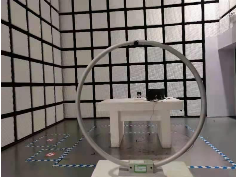
Fig. 1 Radiated emission setup photo(Below 30MHz)
