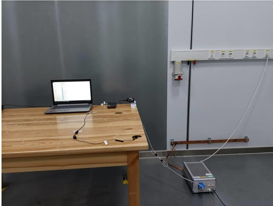
Fig. 3 Power line conducted emission setup photo
