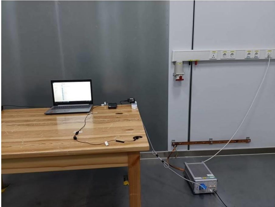
Fig. 3 Power line conducted emission setup photo
