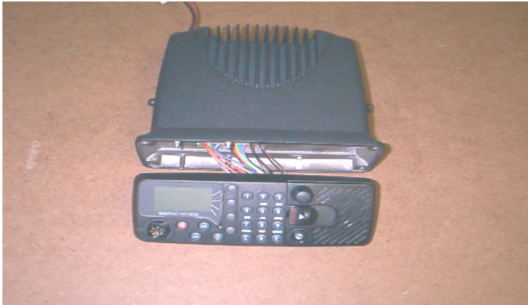
PHOTOGRAPH 12 RD62 showing the Rx/Tx & front panel sections
