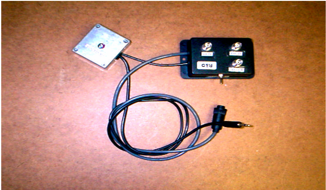
PHOTOGRAPH 14 General view of ptt connection box used during testing
