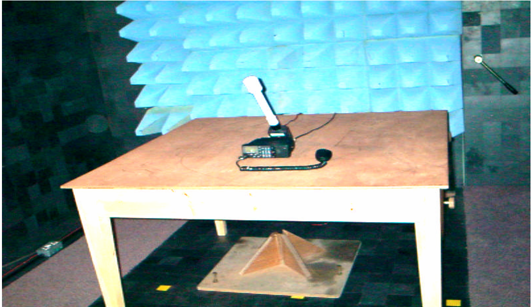
PHOTOGRAPH 4 Close up view of RD62 during radiated immunity test
