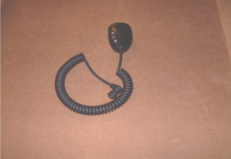
PHOTOGRAPH 8 Front view of RD64 fist-microphone
