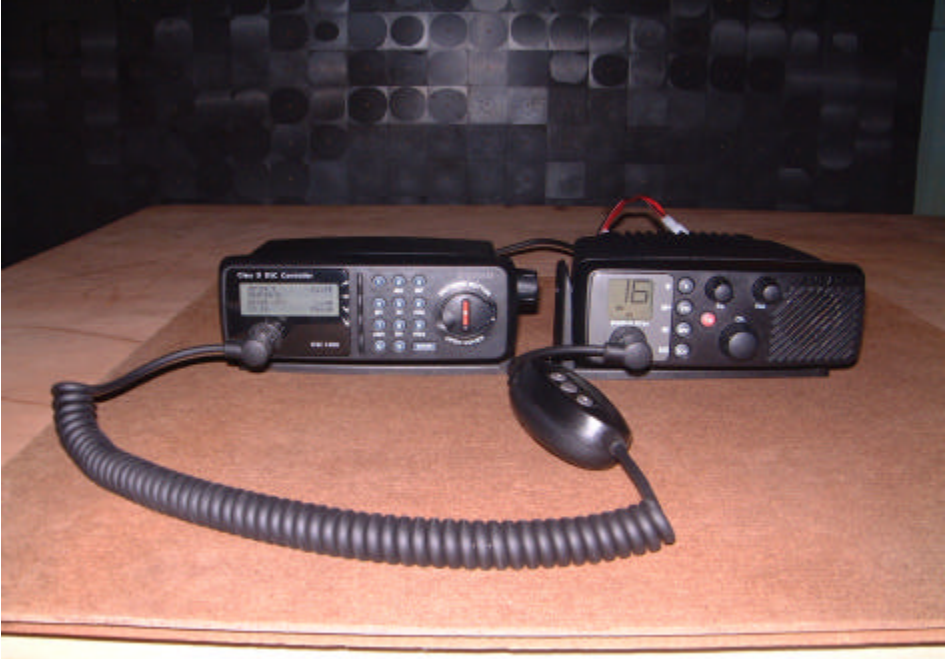
PHOTOGRAPH 3 General view of RD64 radiotelephone with DSC1400 Controller
