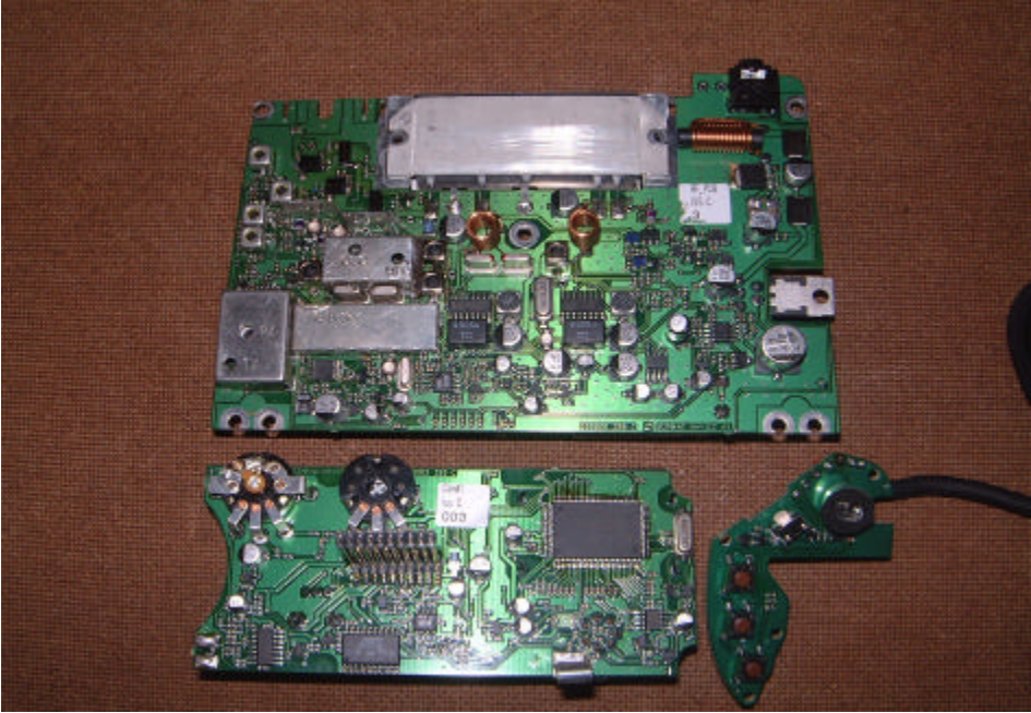
PHOTOGRAPH 6 RT63 Rx/Tx PCB & front panel PCB
