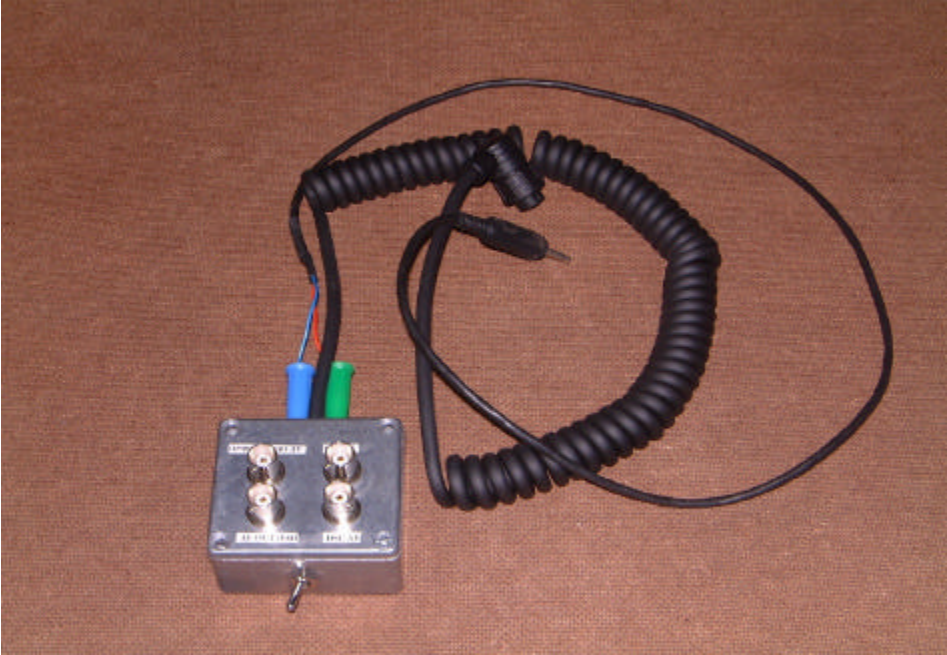
PHOTOGRAPH 7 General view of ptt connection box used during testing
