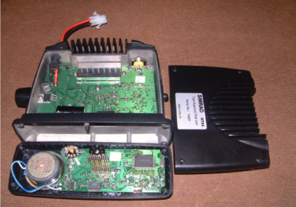
PHOTOGRAPH 5 RT63 showing the Rx/Tx & front panel sections
