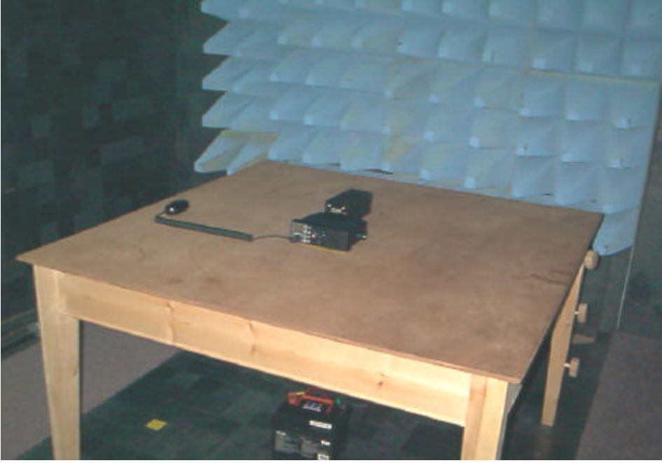
PHOTOGRAPH 2 Close up view of RD64 during radiated emissions test
